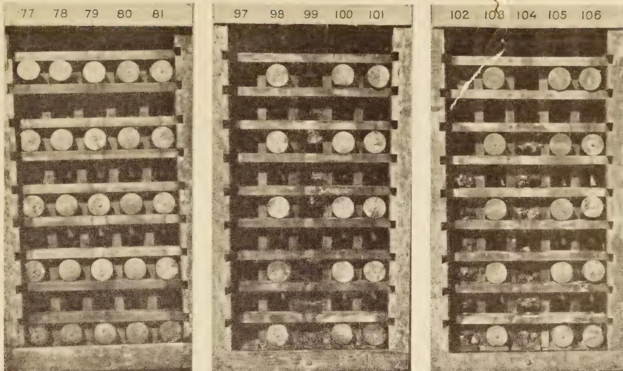
Cylinders cured in steam at 212° F., after six and one-half years in lake
